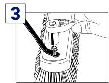
tighten with <sup>5/</sup>16-inch socket
